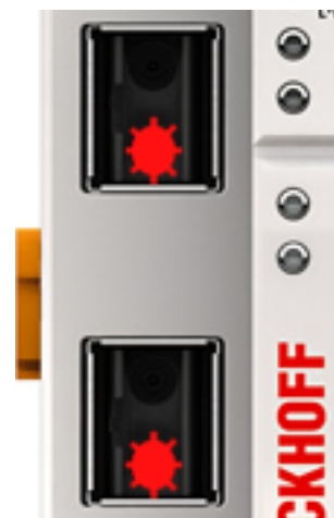
Figure: Transmitter channels in the EK1541
