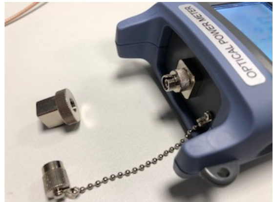
OPM with FC adapter screwed on
