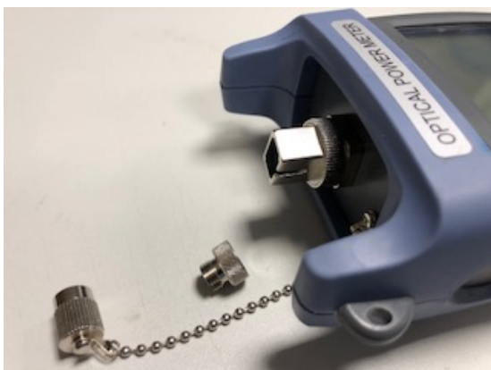
OPM with SC adapter screwed on
