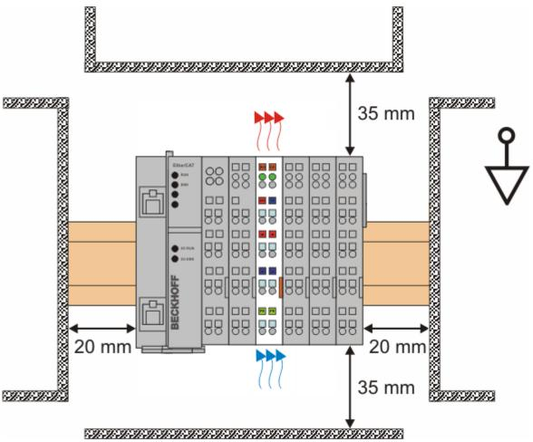
Fig. 30: Recommended distances for standard installation position
