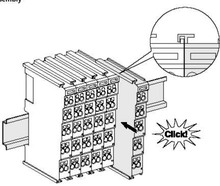
Fig. 23: Attaching on mounting rail
