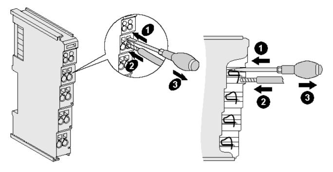
Fig. 29: Connecting a cable on a terminal point
