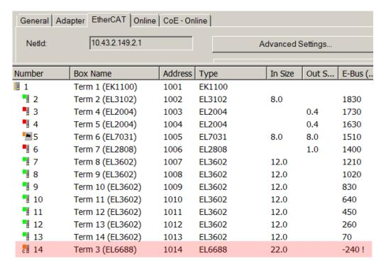
Fig. 141: Illegally exceeding the E-Bus current
