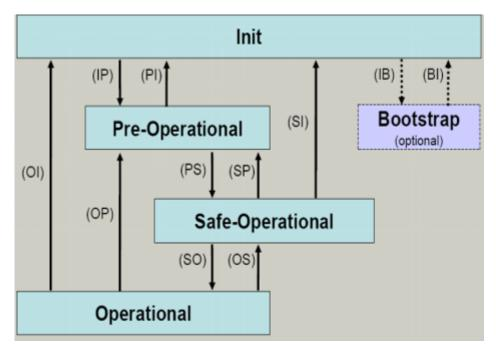
Fig. 21: States of the EtherCAT State Machine
