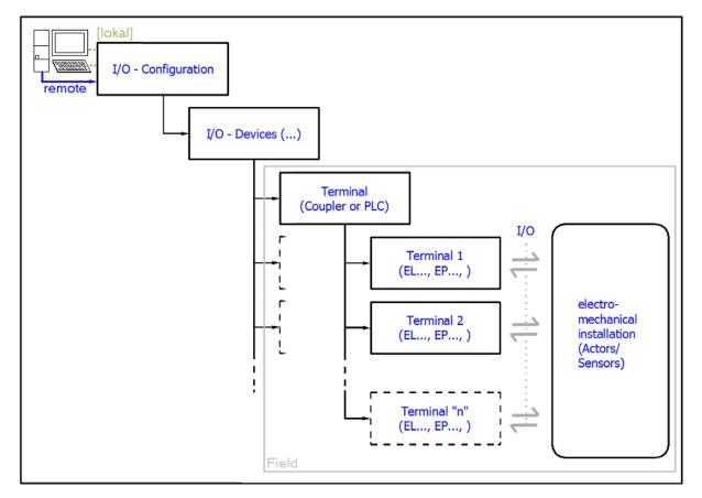
Fig. 34: Relationship between user side (commissioning) and installation
