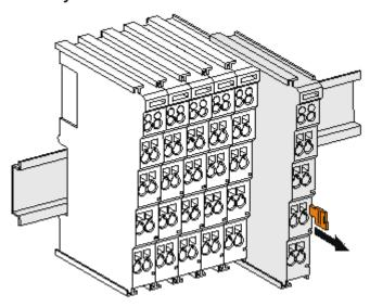
Fig. 24: Disassembling of terminal
