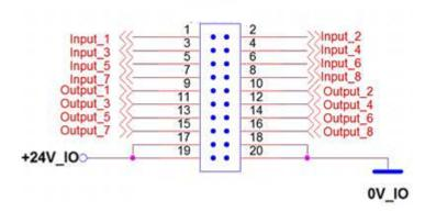
Fig. 12: Pin assignment connector
