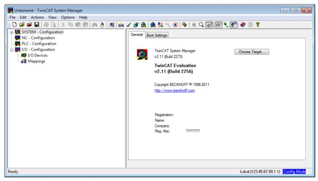
Fig. 36: Initial TwinCAT 2 user interface
