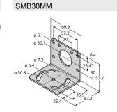
3027162 Mounting bracket, rectangular, stainless steel, for sensors with 30 mm thread, wide holes for accurate alignment
