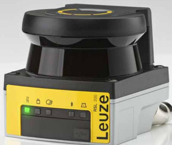
With their dimensions of 80 x 80 x 86 mm, the compact RSL 200 safety laser scanners take up very little space and can therefore be easily and unobtrusively integrated into the machine design. With a range of 3.00 m and a 275° scanning angle, they offer cost-effective solutions for many standard area guarding tasks.
