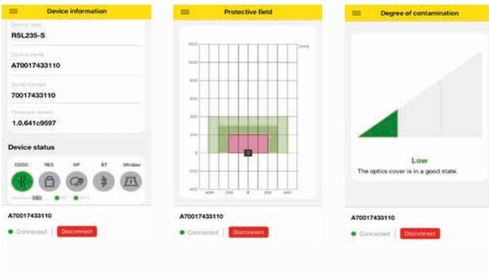
The RSL 200 app enables easy access to status information and diagnostic data via Bluetooth - even if the RSL 200 is installed in areas that are difficult to see or access to the device is restricted. Bluetooth remote access does not affect machine availability. All messages are displayed in plain text and can also be sent directly to Leuze Service if required.
